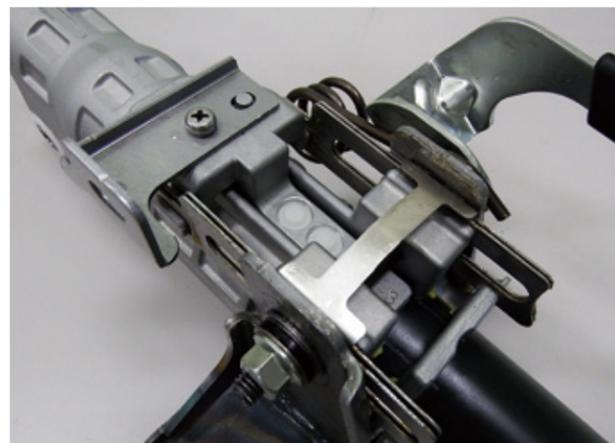
Photo 2 New breakaway mechanism portion
