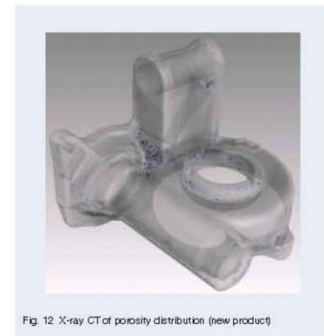
product, the porosity content decreased by 84% and the maximum porosity size decreased by 88% compared with the conventional product. In addition, the porosity content ratio of this developed product is very low compared with the NSK products so far, and it is considered that the quality had also remarkably improved.
