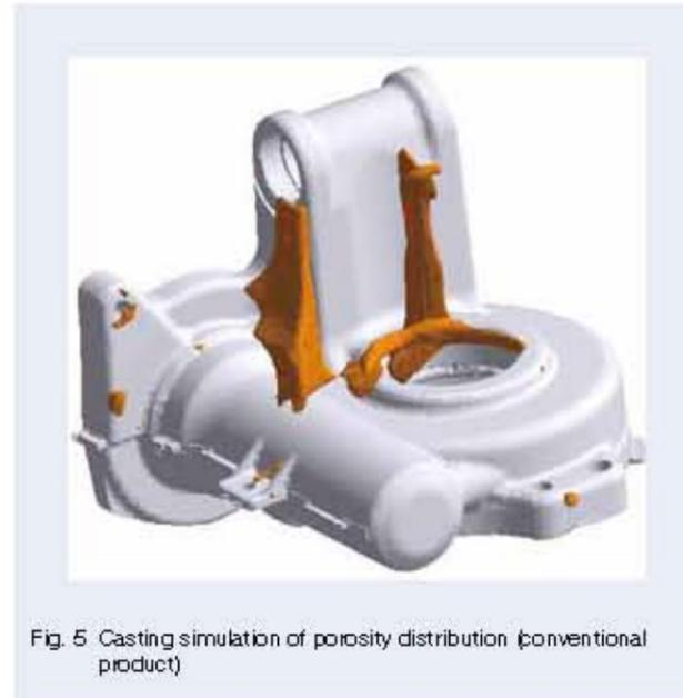
Fig. 5 Casting simulation of porosity distribution (conventional product)
