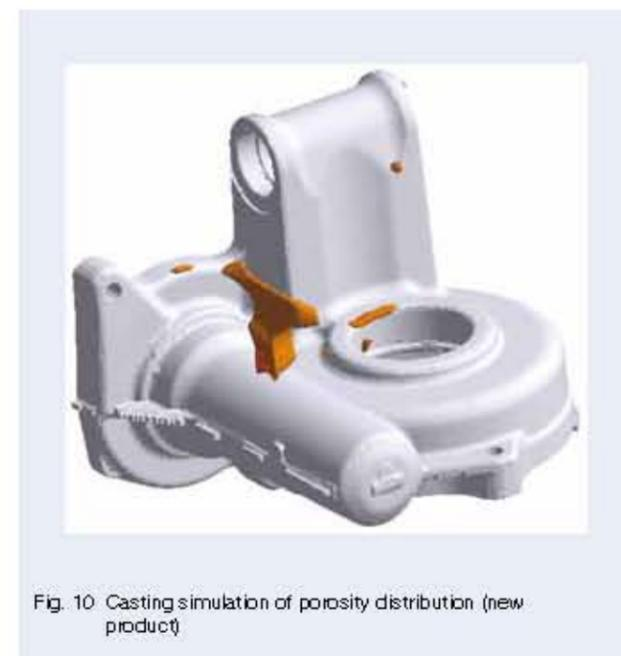
From the comparison with the same simulation result of the conventional product (Figure 6), it is possible to understand that the amount of entrained gas is smaller in the developed product than that in the conventional product, and the range is also reduced in distribution.
