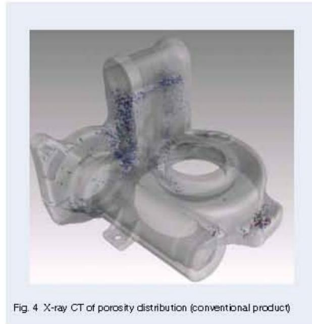
Fig. 4 X-ray CT of porosity distribution (conventional product)
