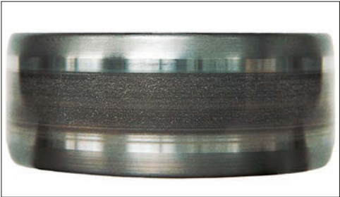
Photo 15-3 Part: Inner ring of a cylindrical roller bearing Symptom: Belt pattern of electrical erosion accompanied by pits on the raceway surface
