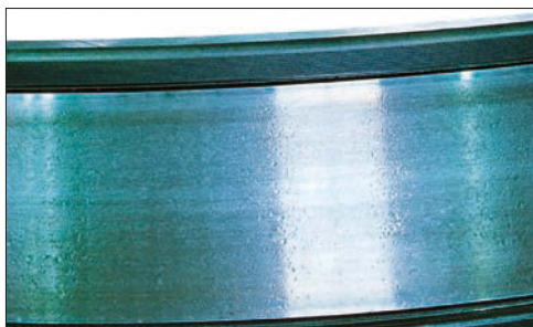
Photo 8-3 Part: Inner ring of a tapered roller bearing Symptom: Small and large indentations over entire raceway surface Cause: Debris caught in the surface
