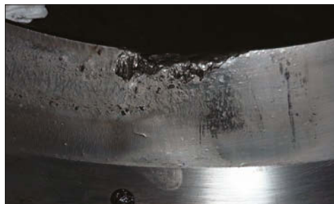
Photo 10-4 Part: Outer ring of a spherical roller bearing (enlargement) Symptom: Combined flaking and wear on the raceway Cause: Insufficient oil film due to poor lubrication led to wear (primary damage) that progressed to flaking (secondary damage)
