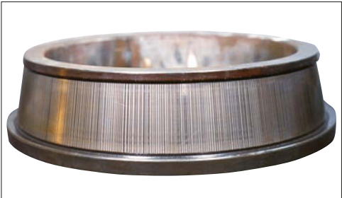
Photo 15-1 Part: Inner ring of a tapered roller bearing Symptom: Striped pattern of erosion on the raceway surface
