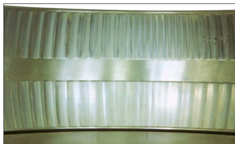
Photo 10-2 Part: Outer ring of a spherical roller bearing Symptom: Wear with a wavy or concave-and-convex texture on loaded side of raceway surface Cause: Entry of debris under repeated vibration while stationary
