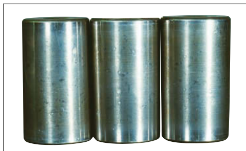
Photo 8-4 Part: Tapered rollers of Photo 8-3 Symptom: Small and large indentations over the rolling surface Cause: Debris caught in the surface
