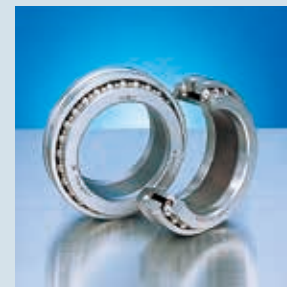
Double-Direction Angular Contact Thrust Ball Bearings NSKTAC D Series 60° contact angle with the highest axial rigidity. Separable type.
