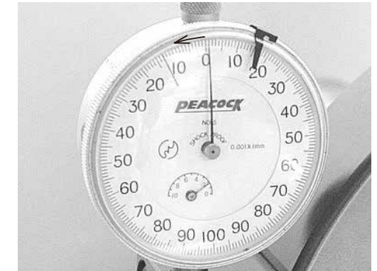
Fig. 1.11 Setting the GN Gauge
