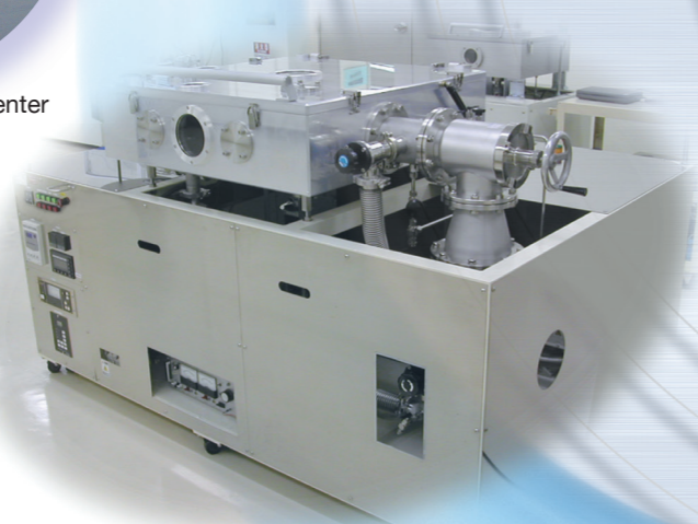
Test rig for bearings for vacuum conditions
