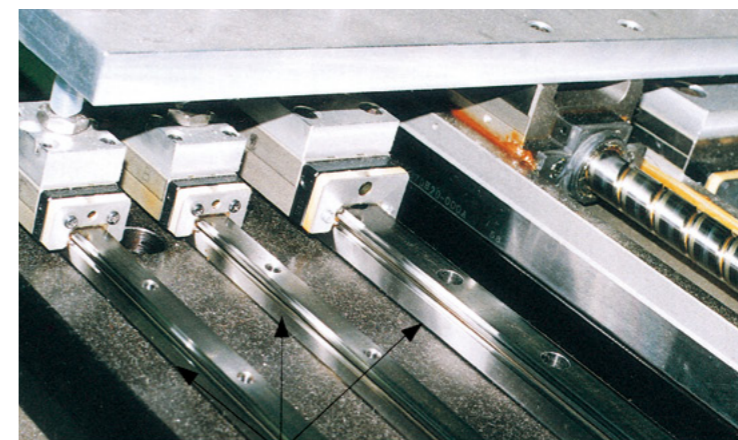
NSK K1 installed linear guide
