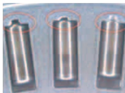
Photo 1. Wear of cage pockets (red circles)
