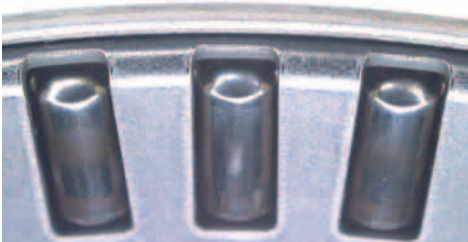
Photo 3 LG thrust needle roller bearings after test
