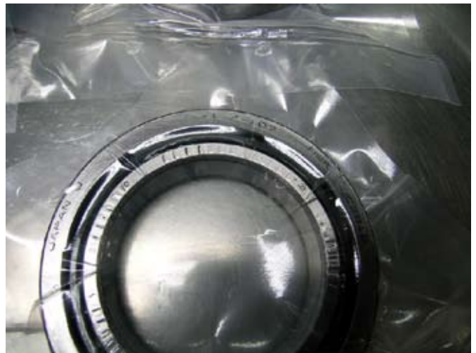
Photo 2 NSK group-wide internal VCI packaging using heat-sealed shrink film
