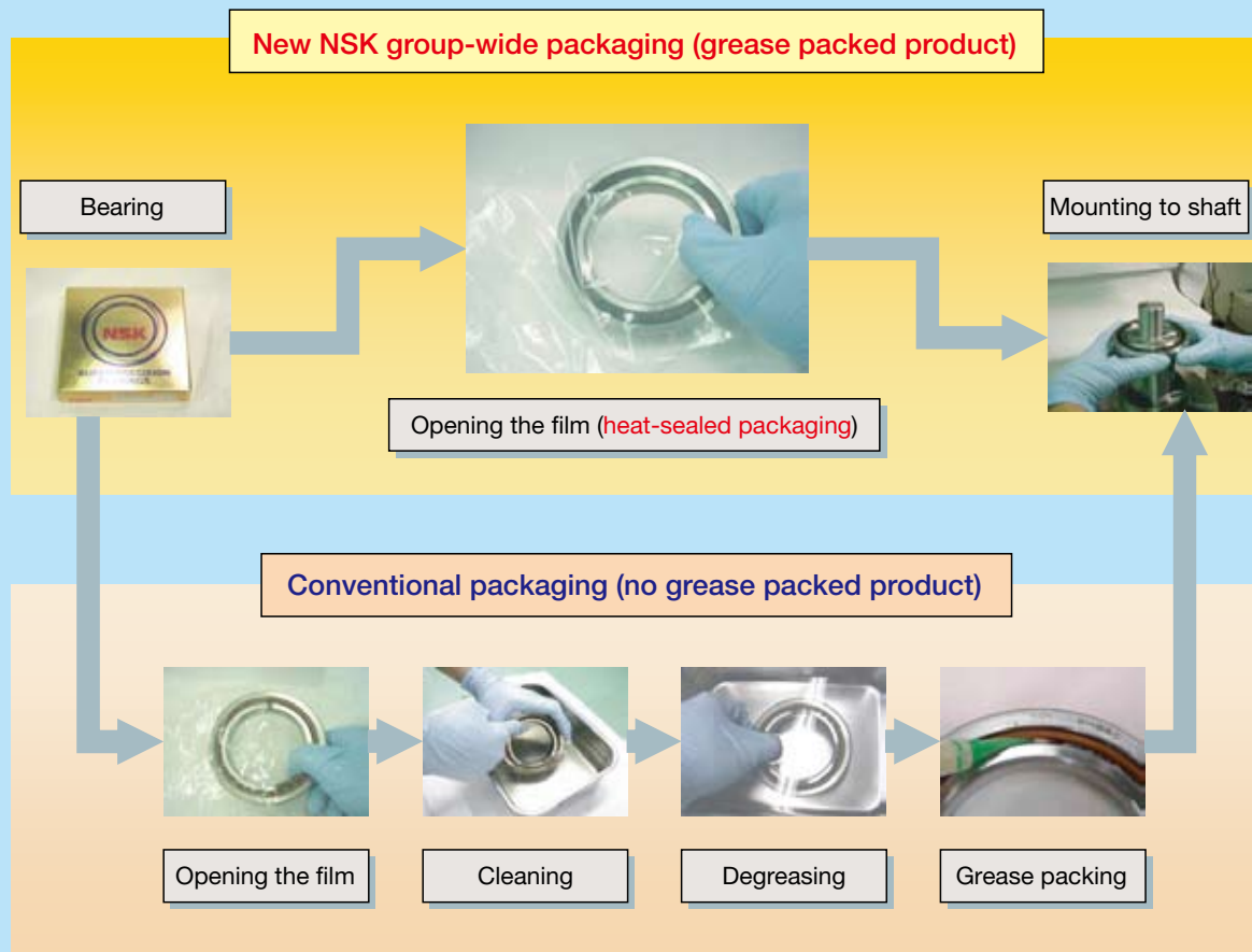
Fig. 1 Comparison of mounting procedures using conventionally packaged bearings (below) and the new standard packaging specification (top)
