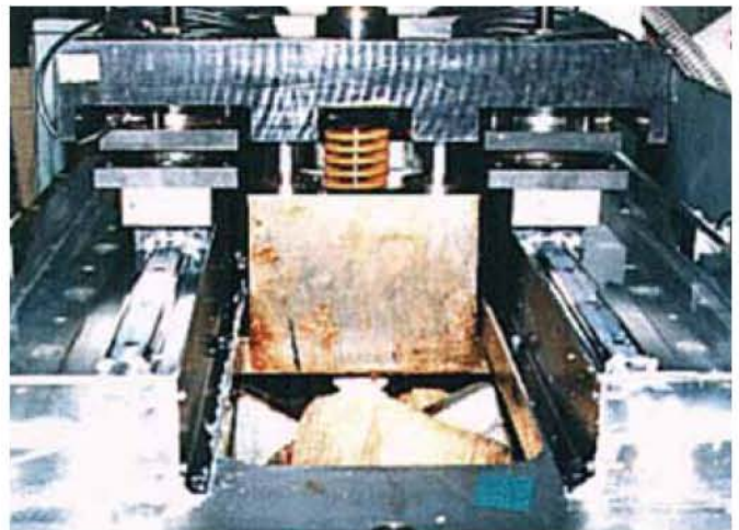
Photo 2 Endurance test of NSK linear guide for food processing equipment and medical devices submerged in water
