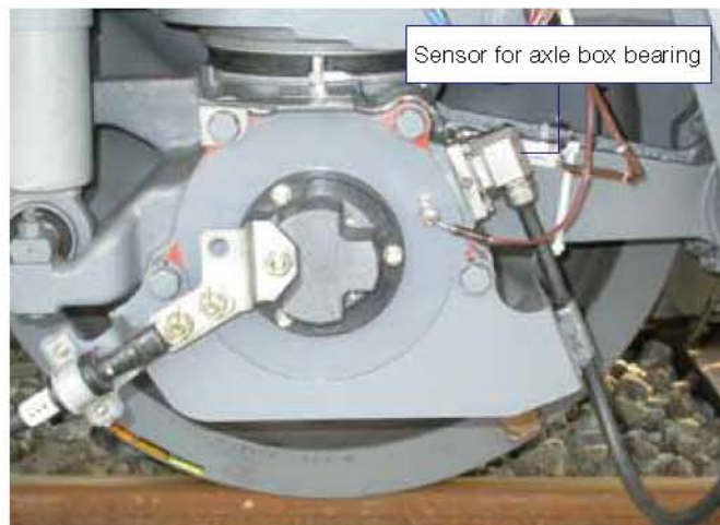
Photo 2 Multi-sensor unit mounted to the housing of an axle bearing for railway rolling stock
