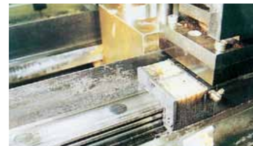
Photo 1 Linear guide undergoing durability testing 5)
