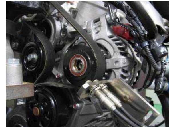
Photo 2 Measuring engine behavior with a clutch pulley mounted to an actual engine
