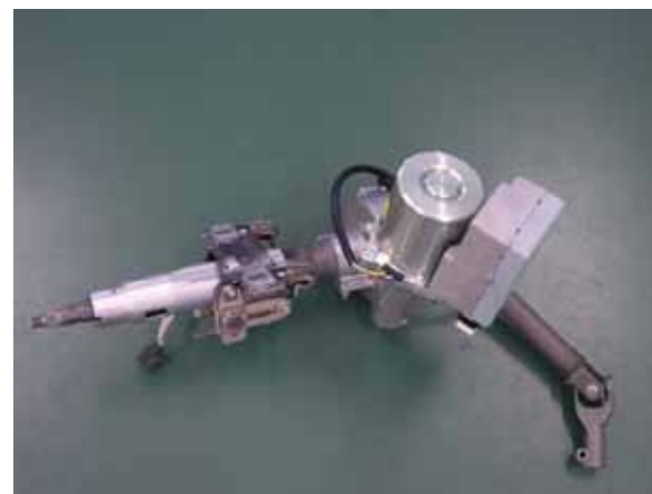
Photo 1 Electric power steering system for excellent on-center steering feel
