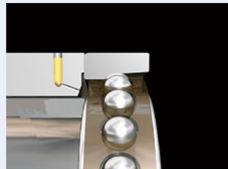
Fig. 5 Conventional oil-air system
