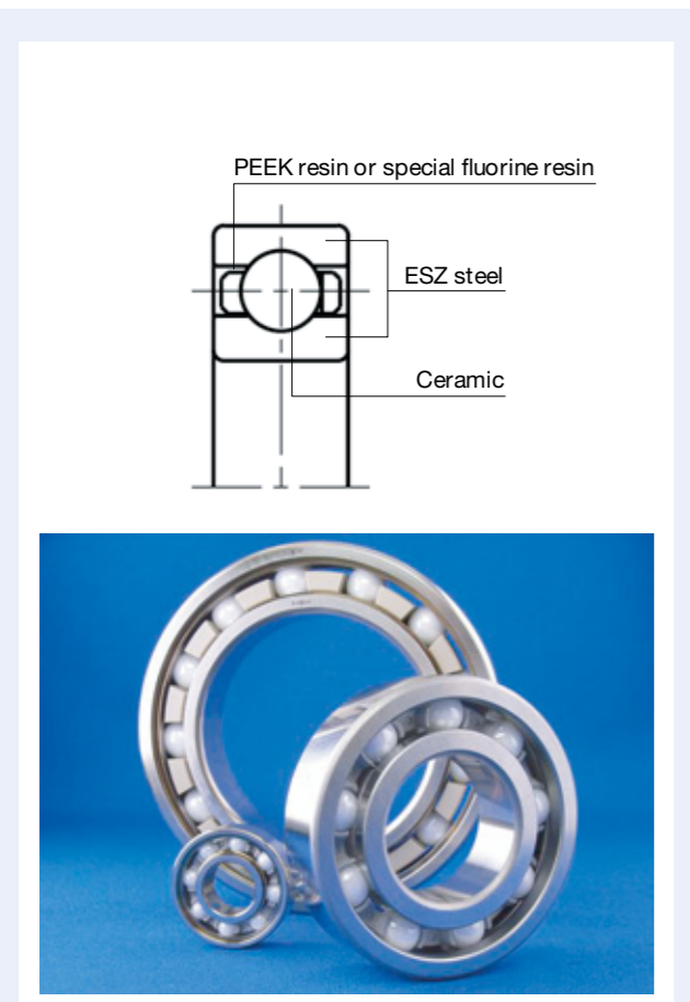
Fig. 1 ESZ bearings made of highly corrosion-resistant, high-hardness stainless steel (deep-groove ball bearing type)
