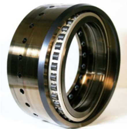
Photo 1 Chemically modified bearing resulting in phosphate surface films (test bearing)
