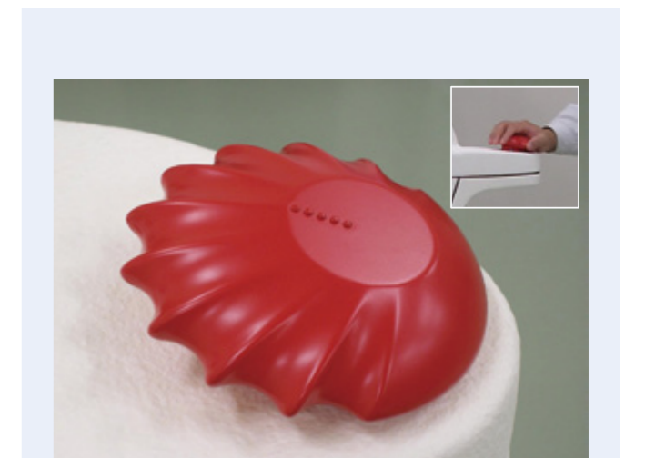
Fig. 2 The grip as an interface between the NWR002 robot and the user
