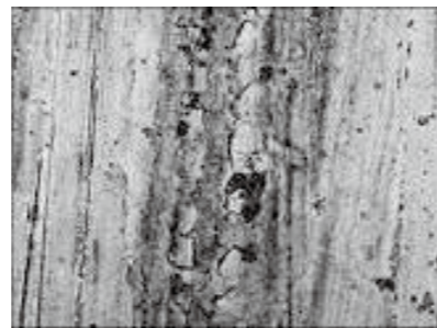
Photo 2 Peeling failure after refrigerant environment testing
