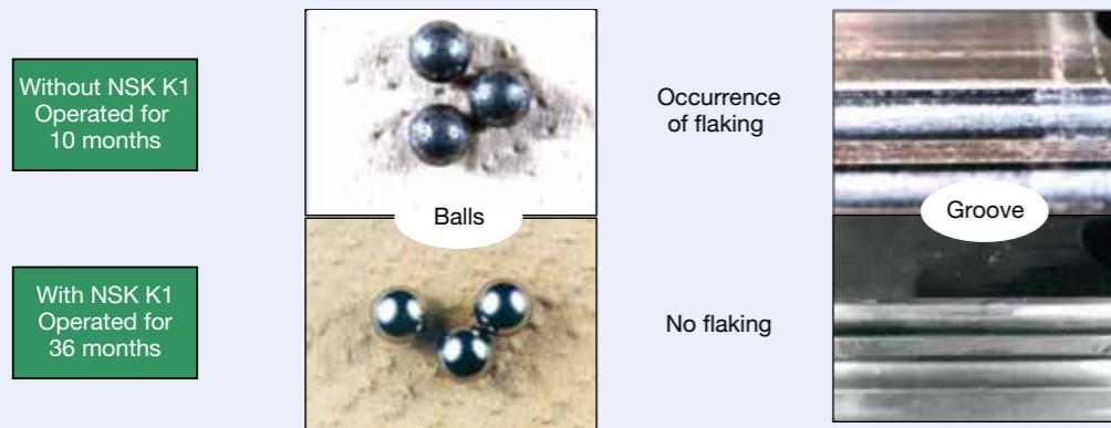
Fig. 10 Example usage results of NSK K1 in the field 6)
