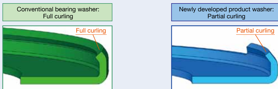
Fig. 3 Partial curling of the new bearing washer and full curling of a previous bearing washer
