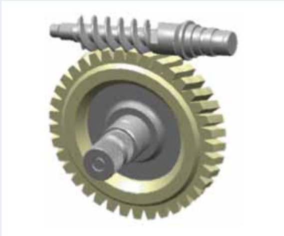
Fig. 3 Worm reduction gear
