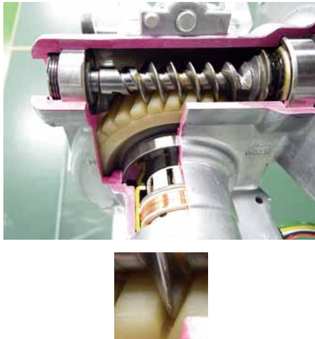
Photo 2 Configuration of the worm reduction gear for EPS
