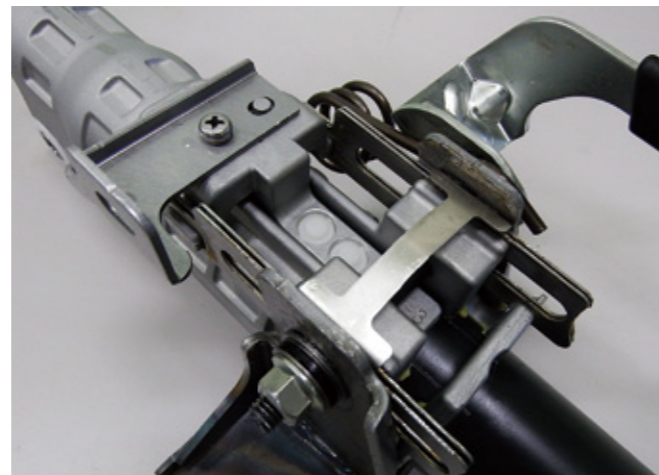
Photo 2 New breakaway mechanism portion
