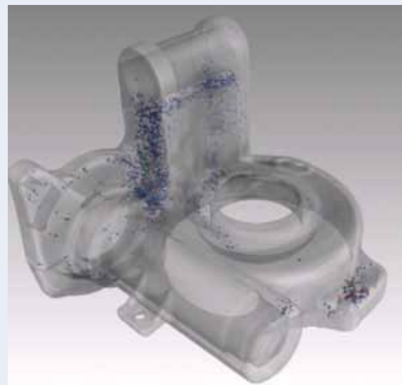
Fig. 4 X-ray CT of porosity distribution (conventional product)
