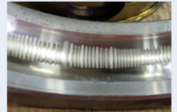
Fig. 10 Electrical erosion on the outer raceway of a deep groove ball bearing
