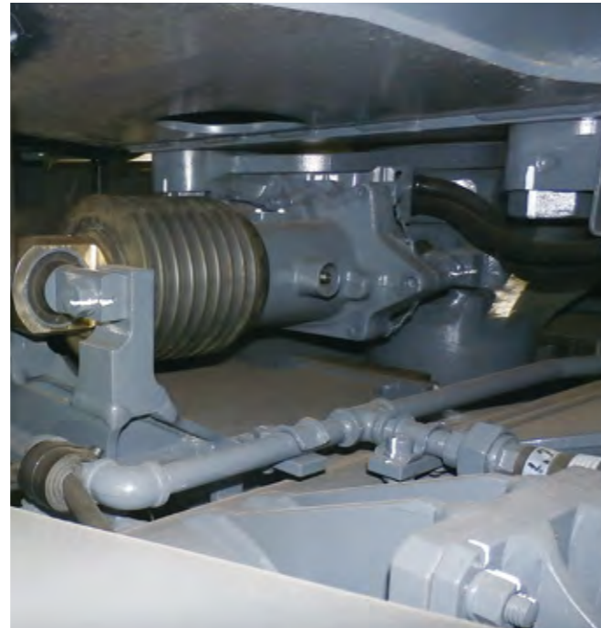
Photo 2 Location of NSK's Vibration Control Actuator (photo: Kawasaki Heavy Industries Ltd.)
