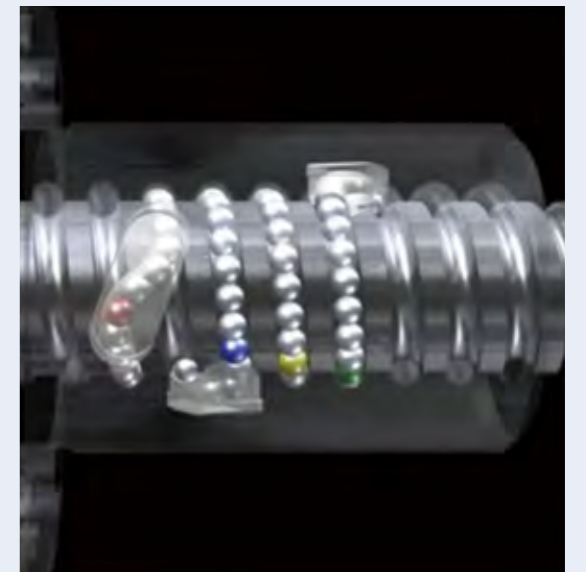
Fig. 12 Proprietary simulation technology for analyzing ball behavior in a nut
