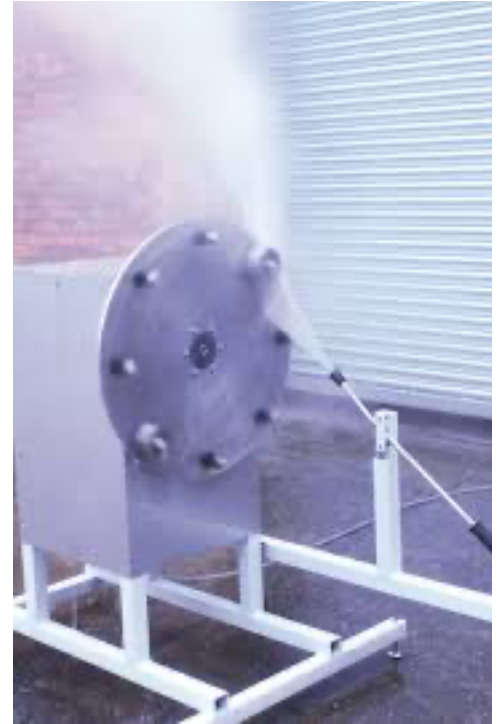
Test rig washing pressure 110Bar
