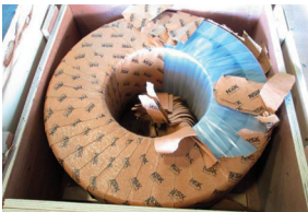
Both images are counterfeit. Incorrect wrapping and no markings.
