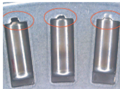
写真1 従来品の保持器摩耗例(赤色円内) Photo 1 Wear of cage pocket
