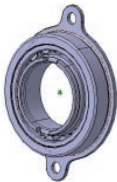
(a) 外輪フランジ付き円筒ころ軸受 (a) Cylindrical roller bearing with outer ring flange
