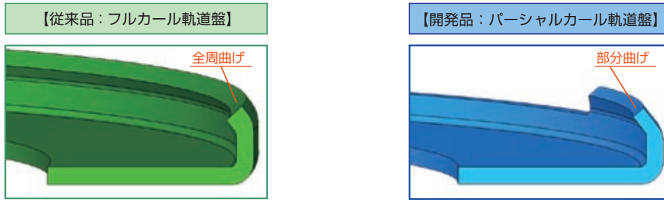
図2 開発品のパーシャルカール軌道盤と従来品のフルカール軌道盤 Fig. 2 Partial curling of newly developed bearing washer and full curling of conventional bearing washer
