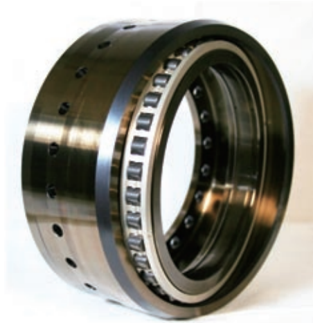
写真 1 りん系改質膜処理を施した軸受(供試軸受) Photo 1 Chemically modified bearing resulting in phosphate surface films (test bearing)
