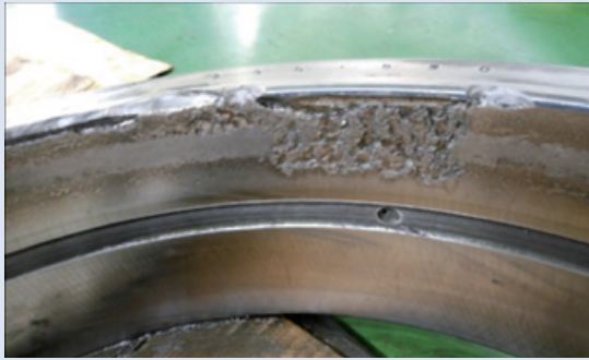
図6 主軸軸受のはく離損傷写真 Fig. 6 Flaking damage on outer-ring of main-bearing
