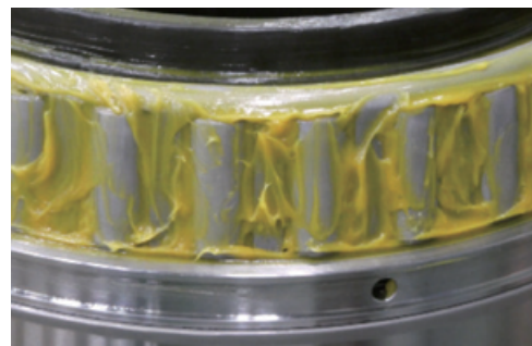
写真2 開発グリース封入状態 Photo 2 Bearing condition with developed grease applied
