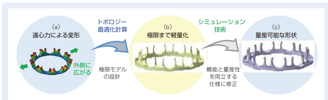
図8 Gen3 保持器の新設計手法 (a) 課題形状 (b) 仮形状 (c) 最終形状 Fig. 8 New design method for Gen 3 cages (a) Issue (b) Working shape (c) Final shape
