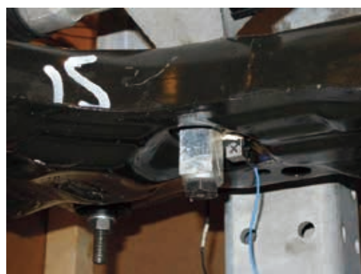
(d) A 3-axis accelerometer on the right hand connection of steering gear housing (No.2).
