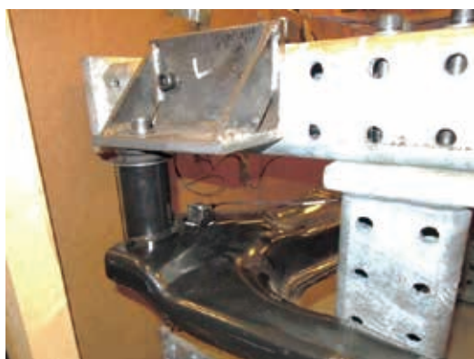
(e) An additional 3-axis accelerometer on the front-right connection of sub-frame (No.12).
