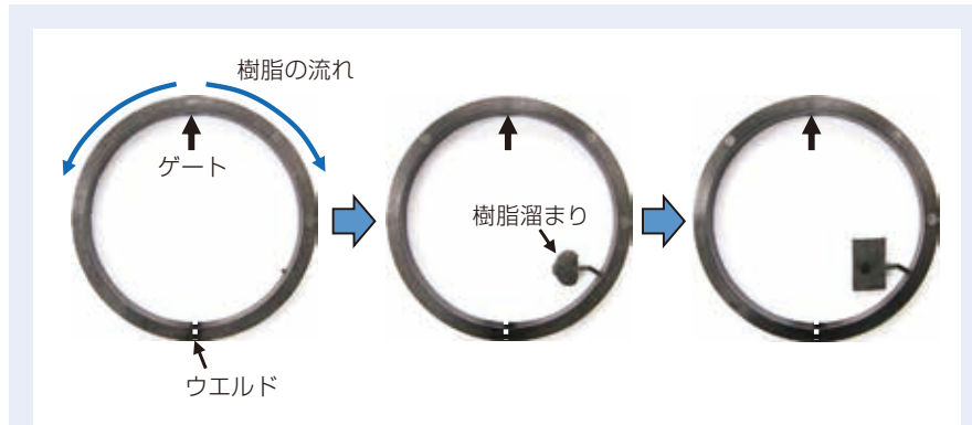
図3 円環試験片の樹脂の充填挙動 Fig. 3 Filling behavior of melt plastic in test piece
